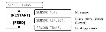
After selecting the sensor type, press the **[PAUSE]** key to show the Printing Method Selection menu.
